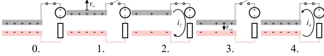
**Fig. 2** The phases of extraction cycle.
