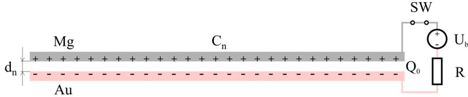
**Fig. 3** The initial charged state.
