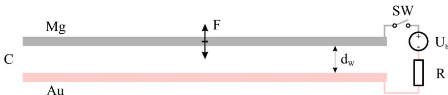
**Fig. 1** Equivalent circuit representation of the parallel plate capacitor made of different metals with movable plates.
